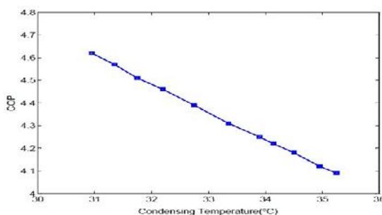
Graph between water cooled condenser temperatures Vs Cop of refrigerator
